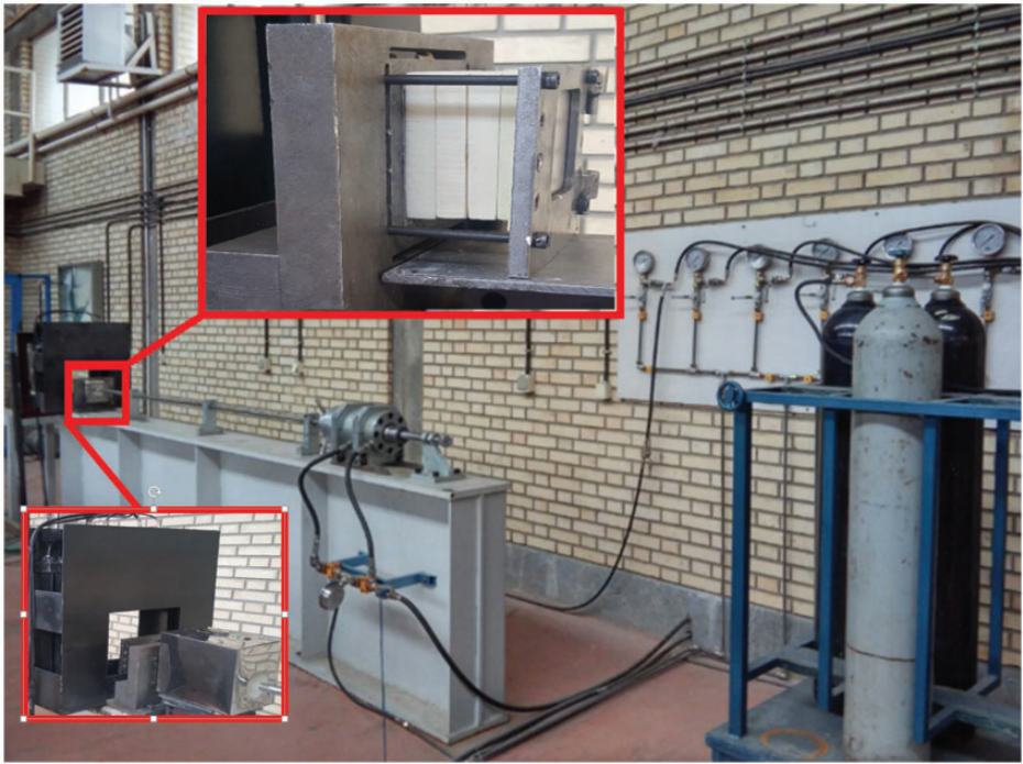
Figure 8. One-stage gas gun and the fixture.
