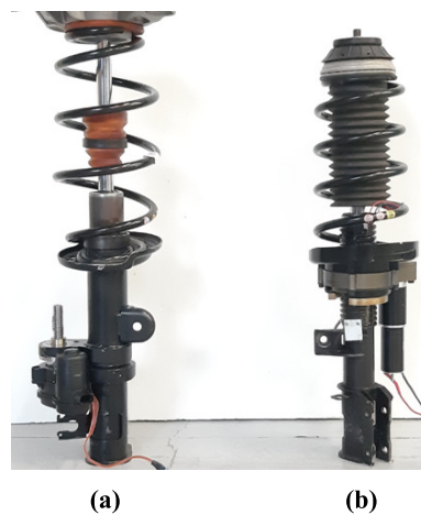
Figure 7. Two height adjustment systems under consideration: (a) eccentrically and (b) concentrically mounted screw systems.
