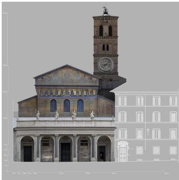
Figure 8. The facade of the Basilica, orthoimage from Structure from Motion (SfM), and 2D model.
