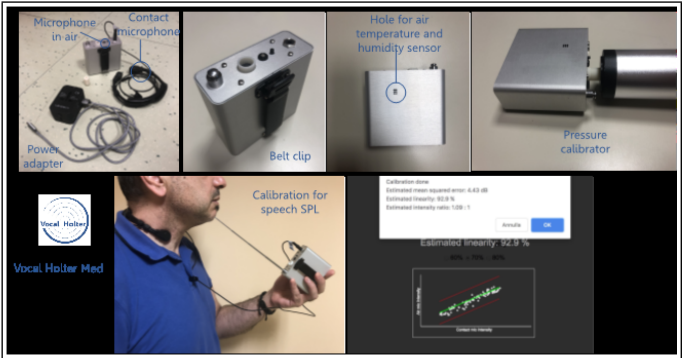
Figure 3. Vocal Holter Med and its calibration procedure for speech SPL.
