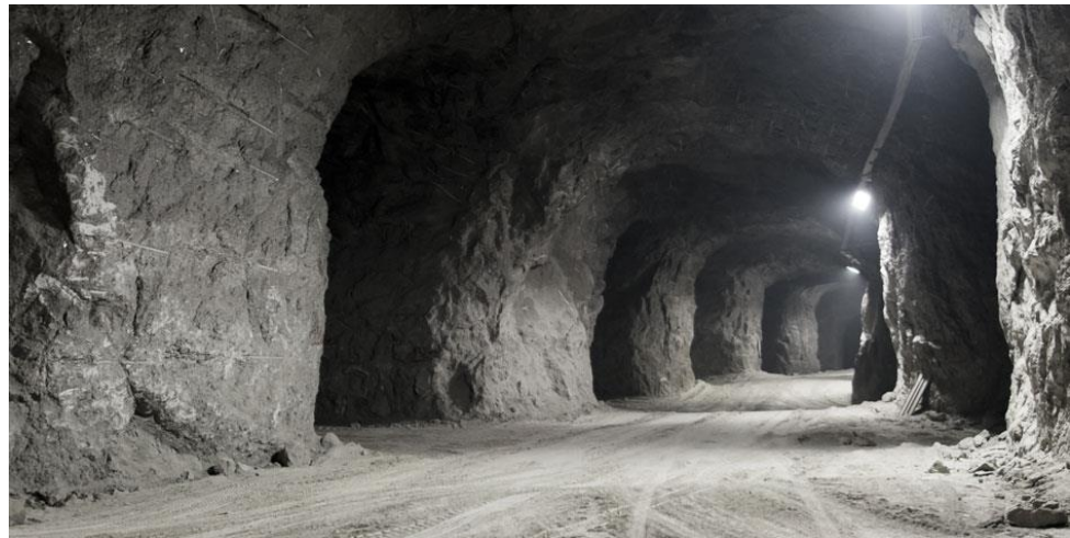
Figure 2. A view of the inside of the Murisengo Underground Quarry with abandoned rock pillars and rooms.
