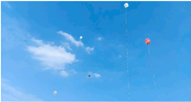
Fig. 12. Experiment with five tethered radiosondes at INRIM on September 29, 2021. Two radiosondes tracked using video camera were marked in red and black.
