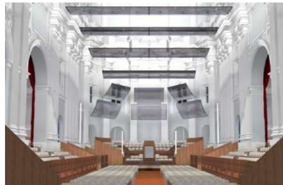
Fig. 9 – Acoustic project design for the adaptation of Santa Lucia's church to an auditorium. Apse side
