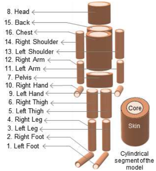
Fig. 1 – Description of segments of the human body in Gagge-2 Core, 16 segment model
