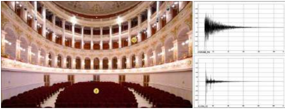
Fig. 8 – Impulse responses measured in the stalls (n 2) and box (2nd order (n 12))
