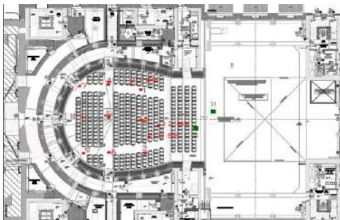
Fig. 10 – Scheme of the equipment location during the acoustic measurements in the stalls of Teatro Galli of Rimini
