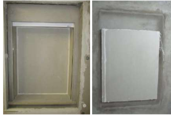
Fig. 4 – Window system for roller shutter “a” – Laboratory test according to ISO 10140 (2021) series standard
