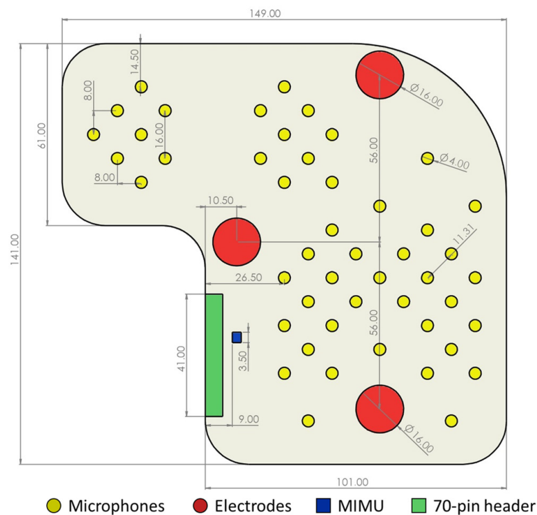
Figure 4. Dimensioned drawing of the multi-sensor array (only relevant dimensions are provided for readability, i.e., dimensions that are either critical for reproducibility or impossible to determine from other dimensions). Dimensions in millimeters.
