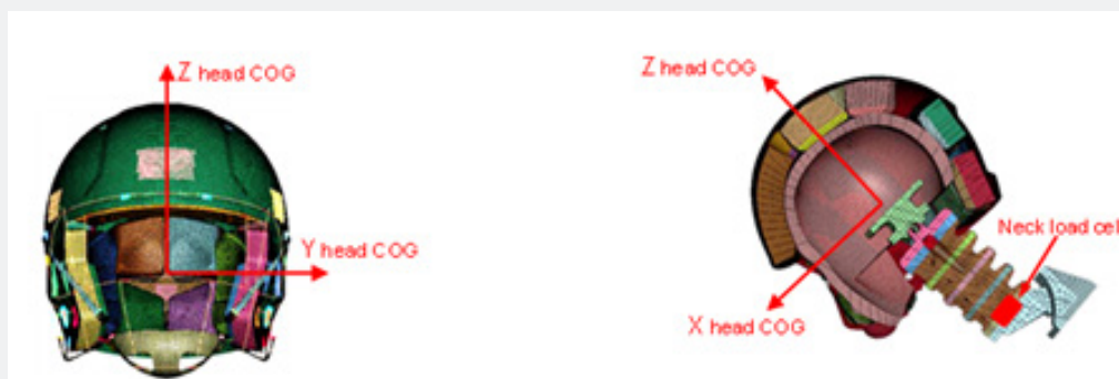
Figure 5. Fitting the Hybrid III headform to the helmet (Left: helmet; right: cross section Hybrid III head in helmet).
