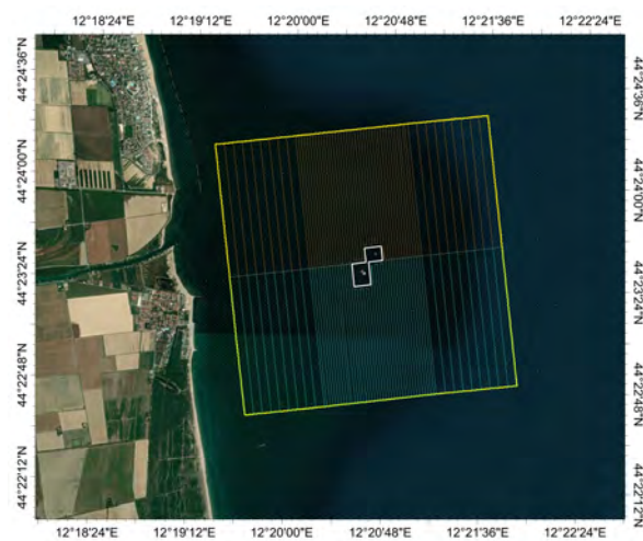
Figure 5. Planned trajectory of the AUV for the survey. The two sub-trajectories are represented by the orange and light-blue lines.
