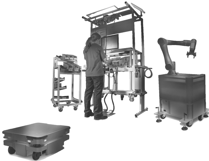
Fig. 3.2 A robot-assisted assembly use case for the presented collaborative framework. The human operator needs to carry out several tasks performed at ad-hoc workstations. The robotic system observes the operator to determine the current process to infer its own desired behaviour.
