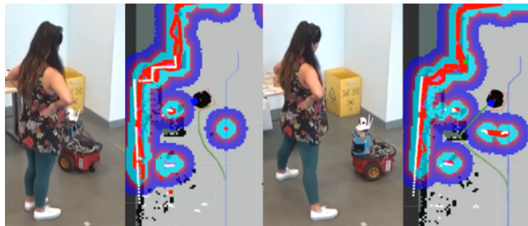
Fig. 2.5 The Sen3Bot human obstacle avoidance behaviour.
