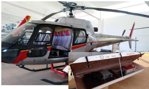
Figure 2. Eurocopter / Airbus AS350 with Litemapper 6800 and particular of EASA certified POD equipped with the LiDAR/Aerophotogrammetric system of CNR-IRPI
