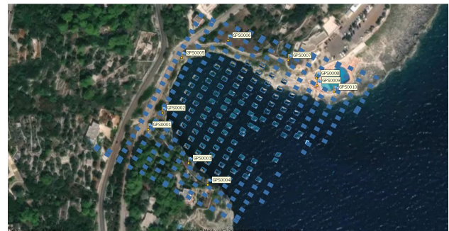
Figure 3. UAS nadiral images acquisition scheme.
