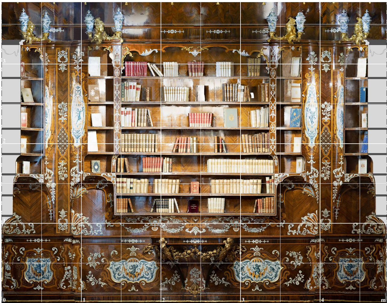
Figure 13. Photogrammetric ortho-image with a metric grid overlapped.
