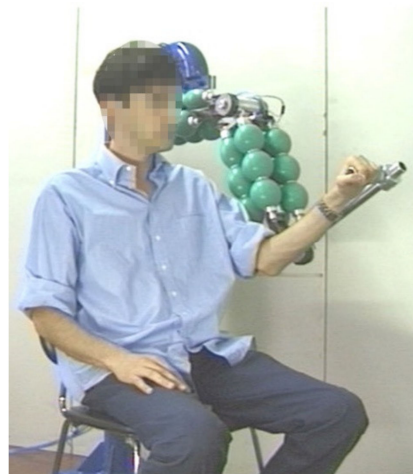
Figure 13. The machine is able to support and drive the limb of the user. The behaviour is smooth thanks to the compliance due to the pneumatic muscle actuators.
