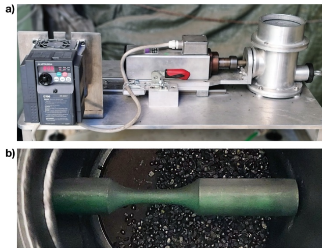
Figure 2. (a) AFB equipment and (b) a sample in the abrasive fluidized bed (AFB)
