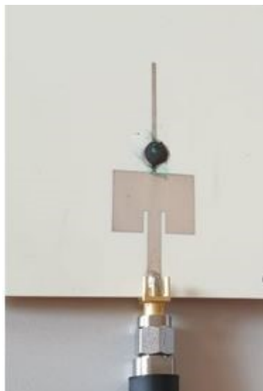
Figure 8. Sensor with drop of HRP.
