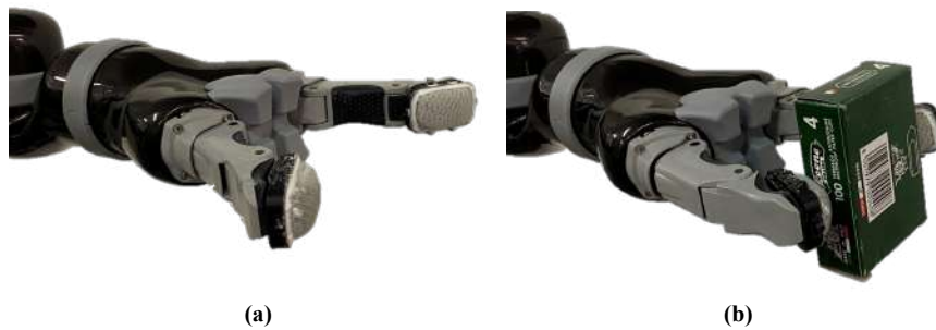
Fig. 1 (a) The proposed soft fingertip mounted on a commercial KinovaGen2 manipulator. (b) Behaviour of the soft fingertip when grasping a generic object.
