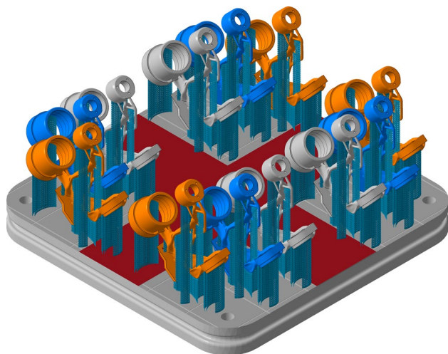
Fig. 7 EOS M 400–4 building platform for GD(1 st ) output (top view dimensions are 400 \times 400 \text{ mm}^2 )
