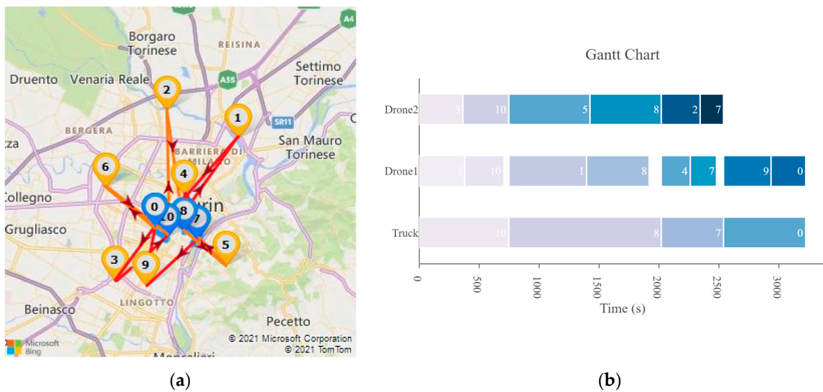
Figure 6. Ad-hoc Method solution representations of Scenario A. (a) mFSTSP tour reported on the map of the operational area, with the paths of the truck (blue), drone 1 (orange) and drone 2 (red); (b) Gantt chart of the mFSTSP solution. The numbers from 1 to 10 in the map and the Gantt chart represent the Customer Node IDs.
