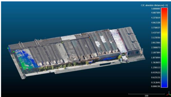
Figure 6. CloudToCloud within a range of 20 cm, emphasizing the drift error in the last part of the MMS point cloud.
