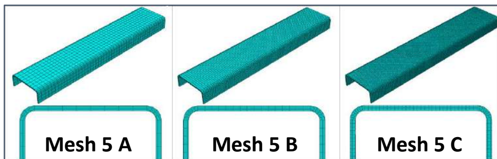
Figure 5. Five elements in the thickness direction: Coarser mesh (Mesh 5A), intermediate mesh (Mesh 5B), and finer mesh (Mesh 5C).
