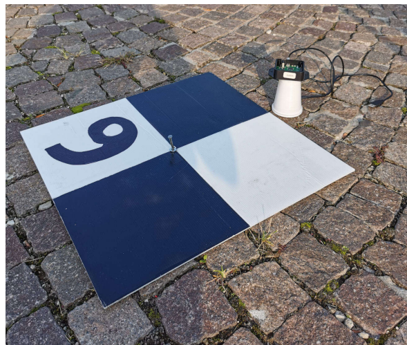
Figure 2. Example of target and Pozyx UWB anchor.
