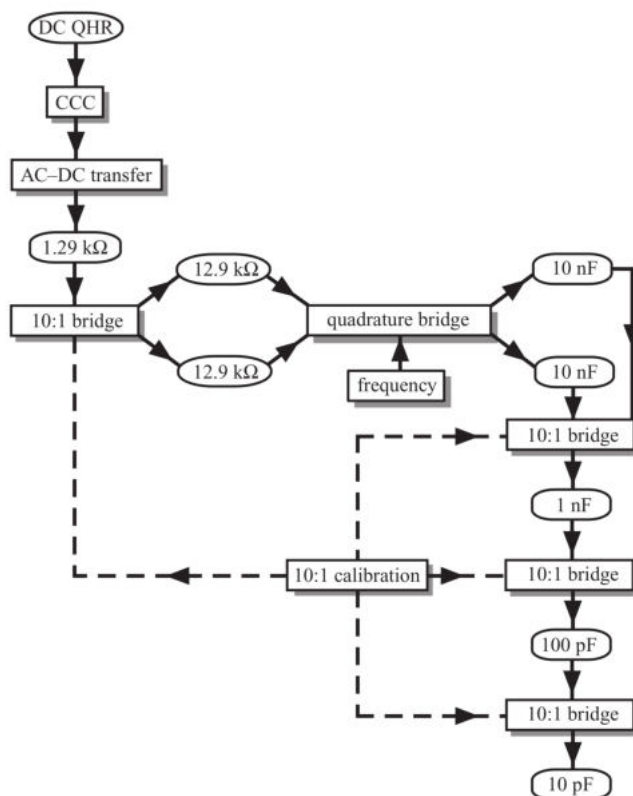
Figure 5.1: Traceability chain for the realisation of capacitance (at 10 pF – 100 pF level) from the dc quantum Hall effect. After Ref. [Sec. 6.37][ ]
