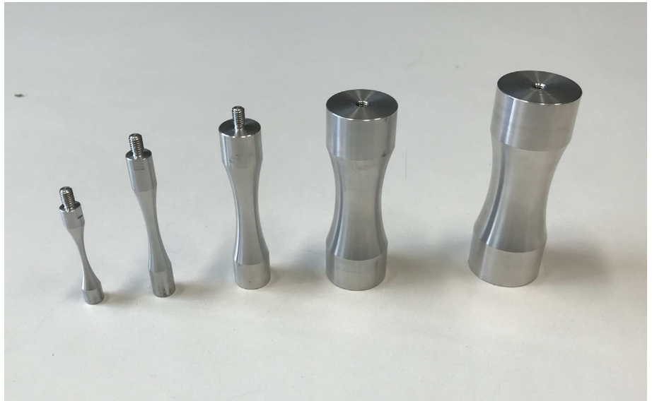
FIGURE 2 The five different tested hourglass and dog-bone specimens. [Colour figure can be viewed at wileyonlinelibrary.com ]
