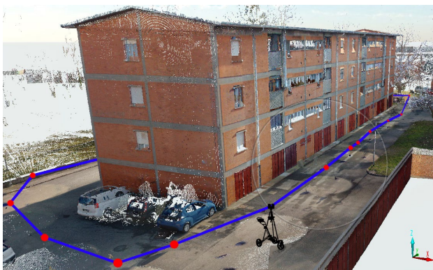
Figure 3. Trajectory followed by the FARO Swift system for the acquisition of the anchor scans for the survey of the analysed building.
