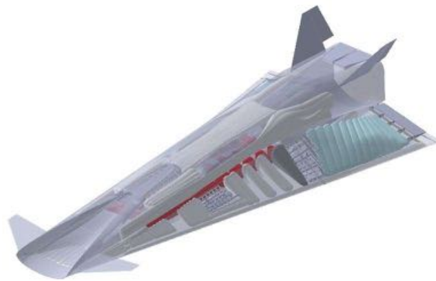
Figure 1. STRATOFly MR3 Vehicle layout with integrated systems.
