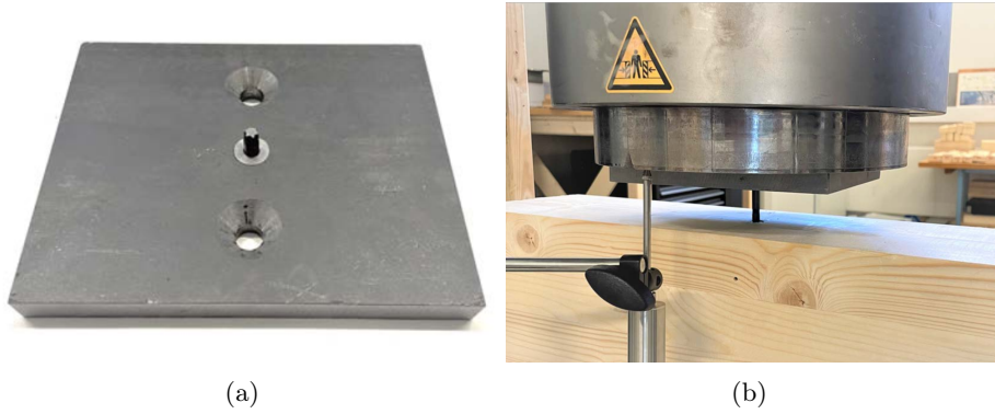
Figure 4: Setup of specimen with height 540 mm in ZwickRoell Z1200-Steel plate used for Torx tests- Setup of Torx test.
