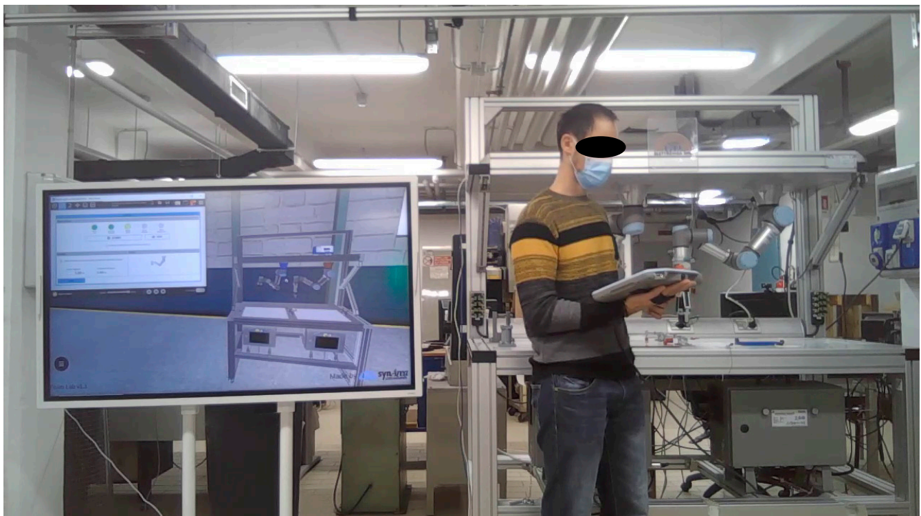
Figure 2. VR replica of the dual arm assembly station complemented with additional information.
