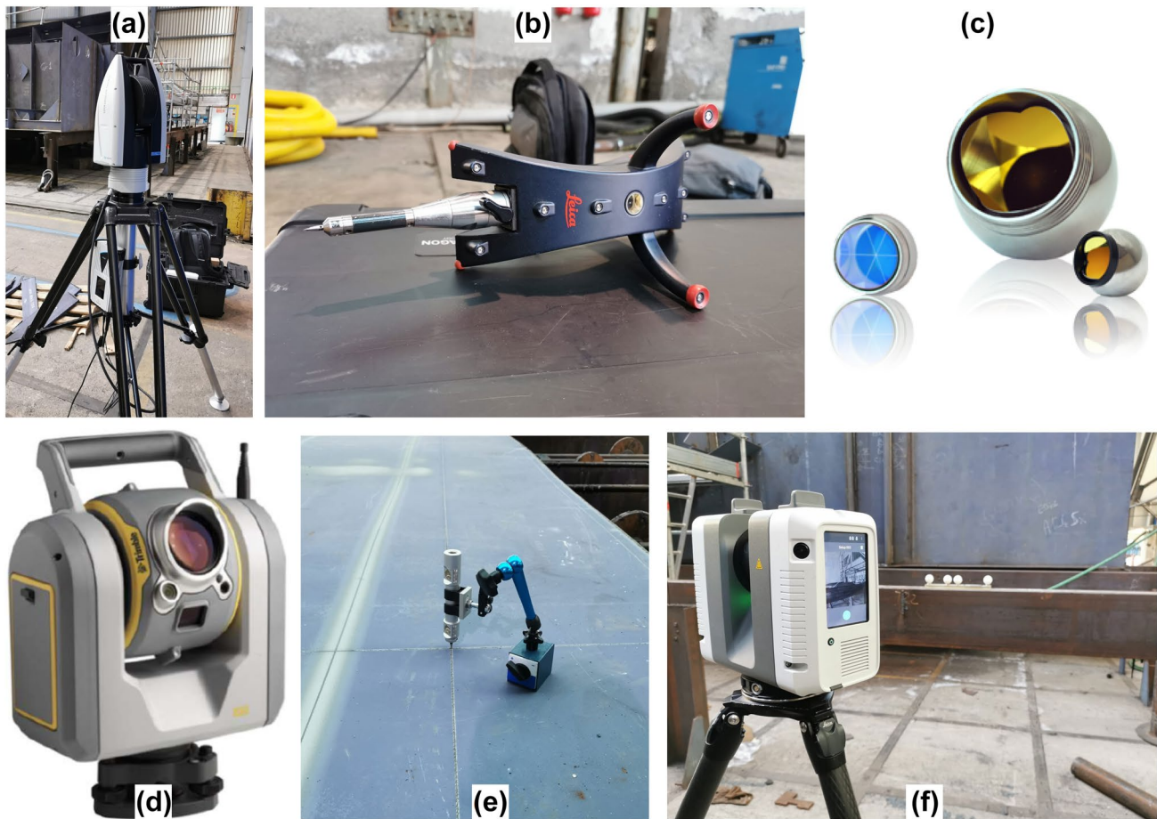
Fig. 1 Measuring instruments and accessories in use: a Leica Absolute Tracker AT960 with b T-Probe and c SMRs of various types (12.7 mm and 38.1 mm diameter), d Trimble SX10 scanning total station with e mini-vector accessory, and f Leica RTC360 scanner
