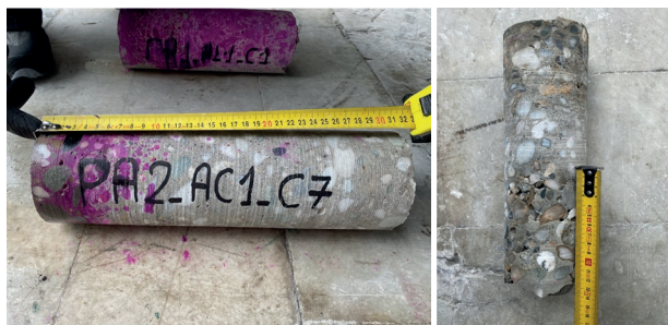
Figure 10 | Sample in the portion of the arch presumably made with Type 680 concrete (on the left), and a sample in the portion of the arch presumably made with Type 500 concrete.
