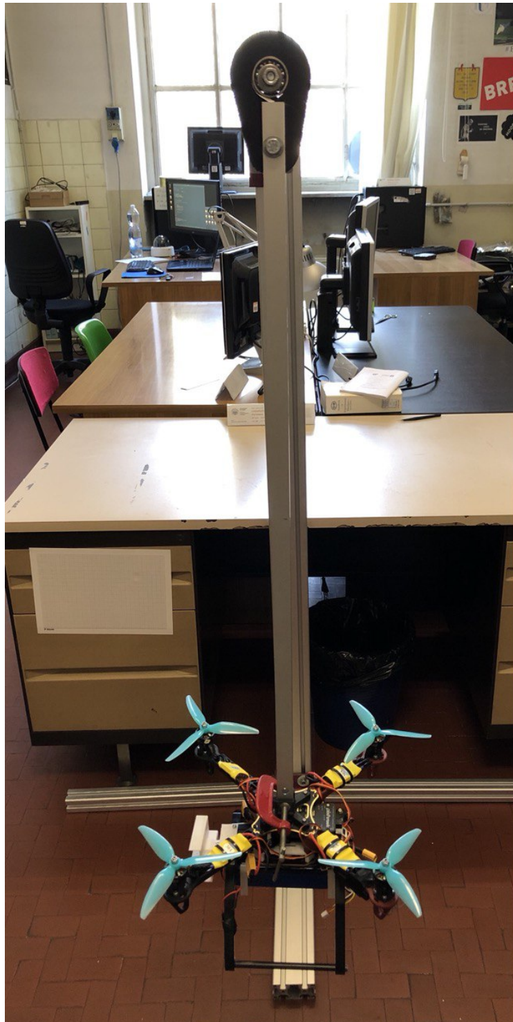
Fig. 2.13 Pendulum employed to measure I_x and I_y .
