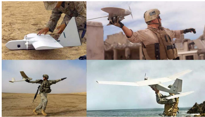
Fig. 1.13 The RQ-14 (top left), WASP (top right), Puma (bottom right) and the RQ-11 (bottom left), [147].
