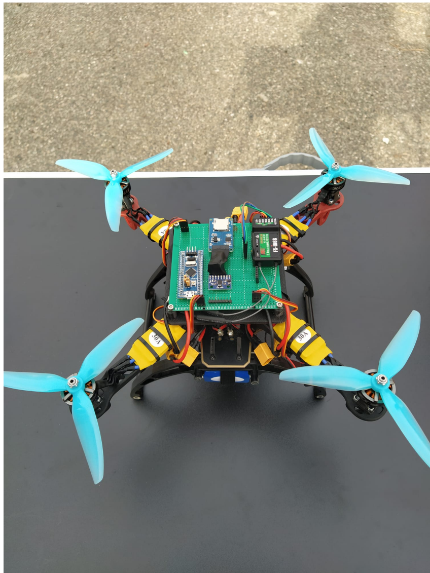
Fig. 2.14 Flight set-up: the quadcopter and the developed Flight Controller.
