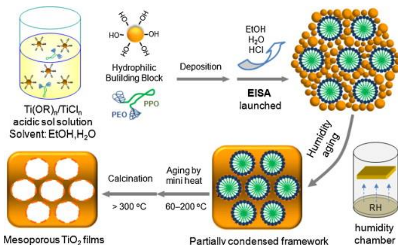
Figure 4.5 Schematic representation of EISA process for the synthesis of highly organized mesoporous TiO 2 films. Adapted with permission from [32]; Copyright 2011 Elsevier
