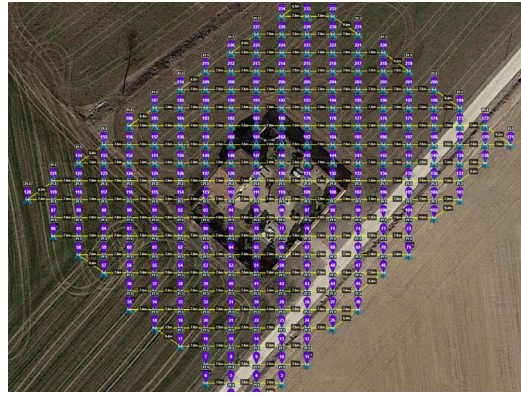
Fig. 5 - First mission. On the left, mission imported to the Litchi app; on the right, alignment of the shots in Agisoft Metashape and representation of each point by means of a reliability gradient.
