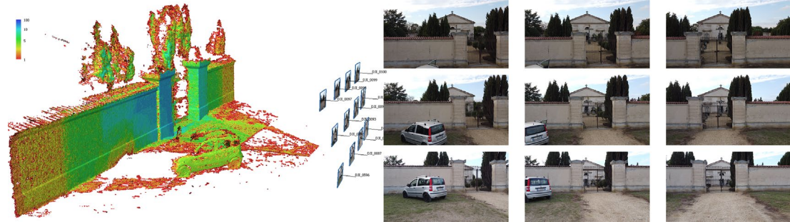
Fig. 7 - Third mission. On the left, alignment of the shots in Agisoft Metashape and representation of each point by means of a reliability gradient. On the right, some frames in which there is an obstacle that generates unwanted portions of the cloud.
