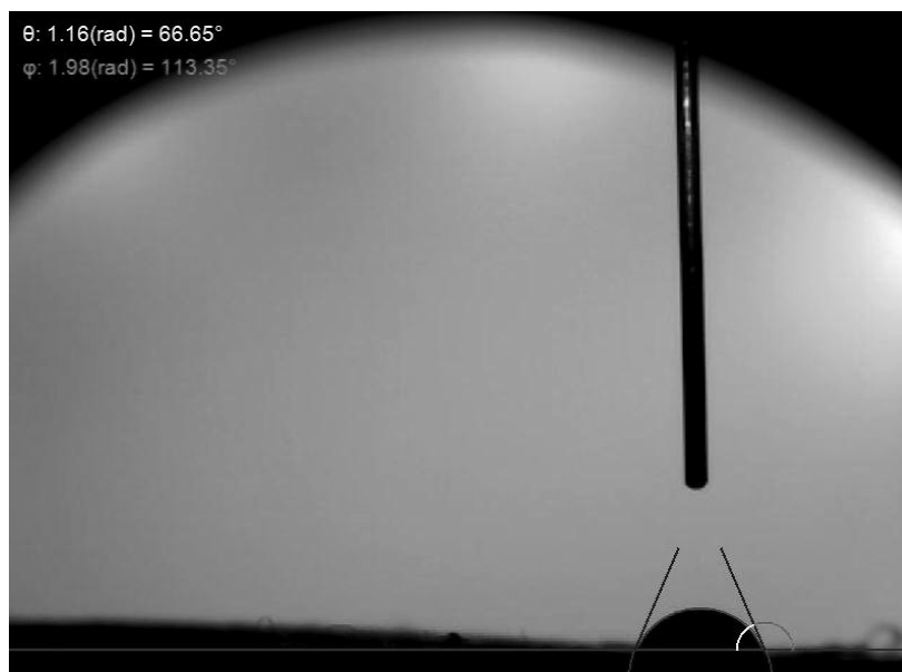
Figure 7. CS-CQD-TiO 2 -GO electrospun nanofibrous mat hydrophilicity. The angle \theta (WCA) is equal to 66.65°.
