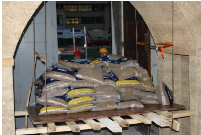
Figure 3: Structural testing of the hemp lime vault
