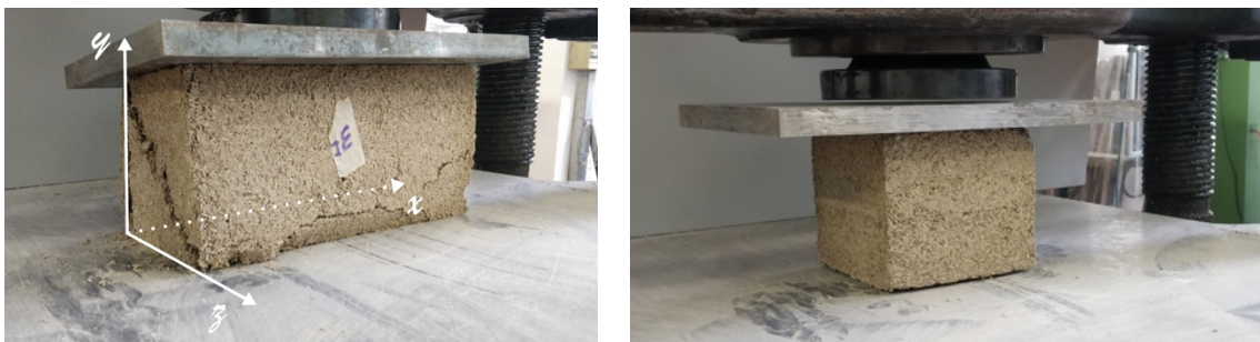
Figure 12: Compression tests of brick and cube samples
