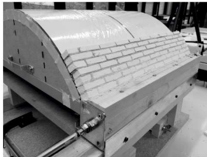
Figure 4: testing device of the barrel vault (a), axonometric exploded view of the centring (b), radial vault during construction (c) and after centring removal (d)
