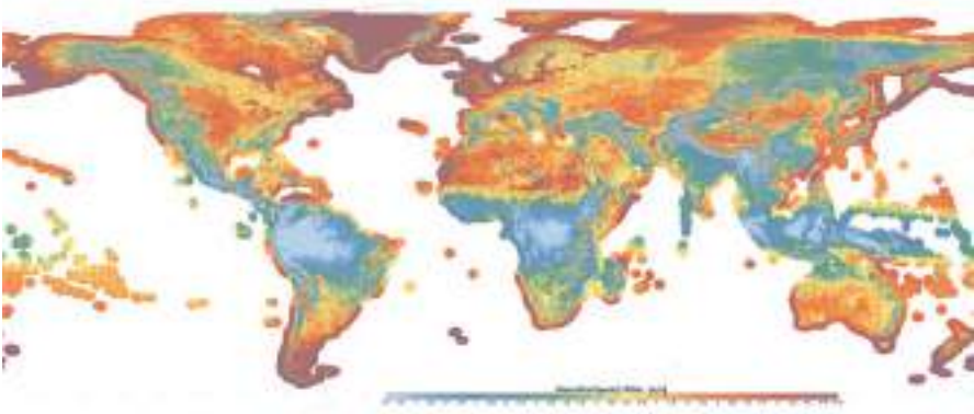
Fig. 10.2 The global wind energy potential shown as mean wind speeds 100 m above ground. (Source: Global Wind Energy Atlas 2019)
