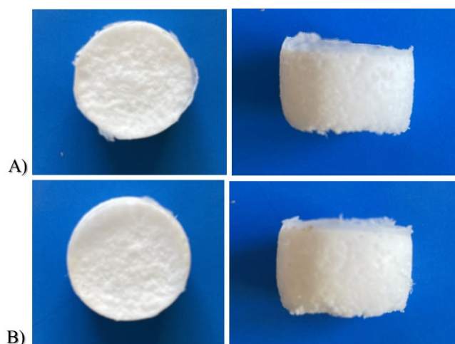
Figure 1. Representative images of the general aspect of the PCL-based scaffolds: pure PCL (A) and 30% EO-added PCL (B) samples with NaCl.
