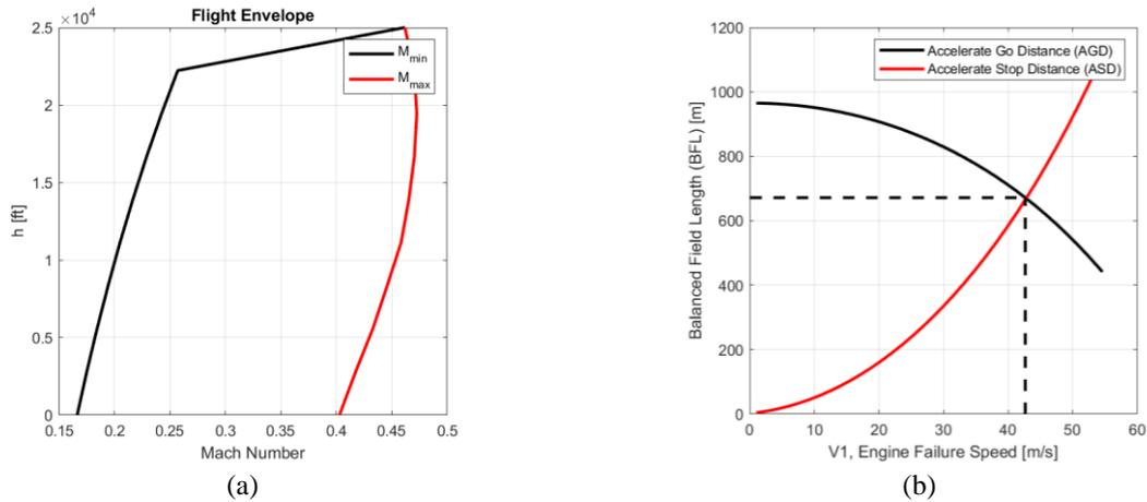
**Fig. 6. Aircraft envelope and balanced field length.**
