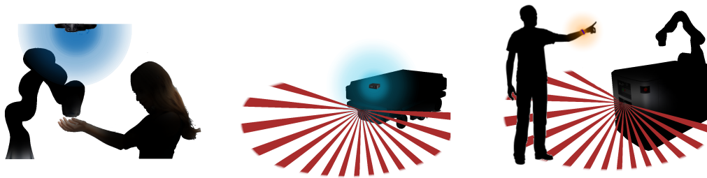
Fig. 7.2 Relevant sensors for HRP within the industrial context. Vision sensors are highlighted in blue, safety laser scanners rays in red, and wearable sensors in orange.
