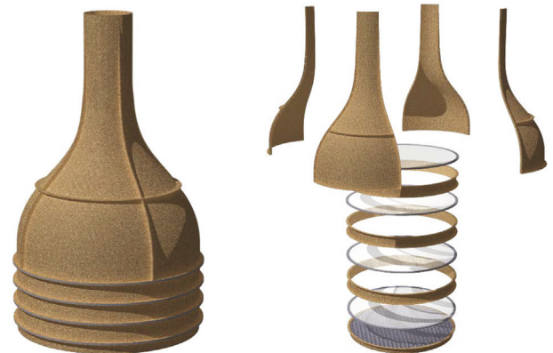
Fig. 2. Detail of the A-tunnel contraction and flow conditioners inside it.
