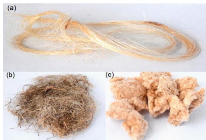
Figure 4. Natural fibers are available in different forms: (a) strands, (b) staple, (c) pulp. Reprinted from ref. [48] with permission of Elsevier Ltd., 2015.
