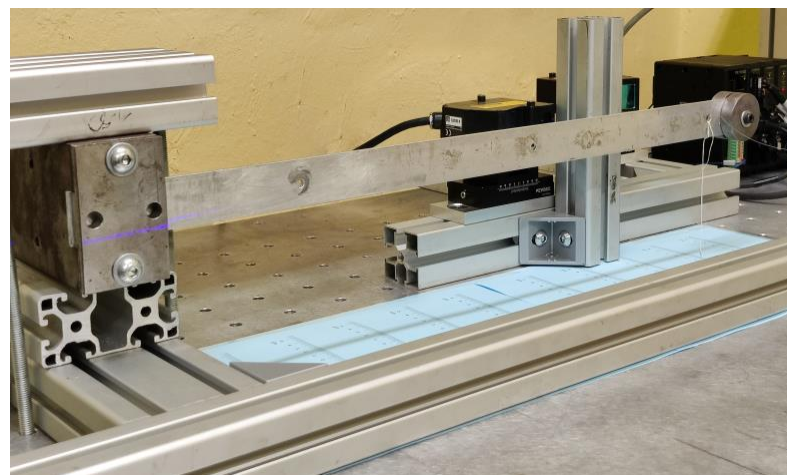
Figure 1. Euler–Bernoulli cantilever beam.
