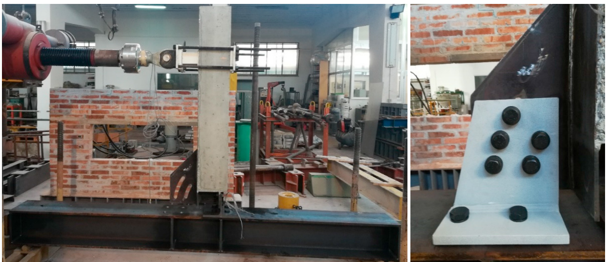
Fig. 8. (a) specimen of the innovative beam-column joint endowed with friction dissipative device; (b) detail of the friction dissipative device.
