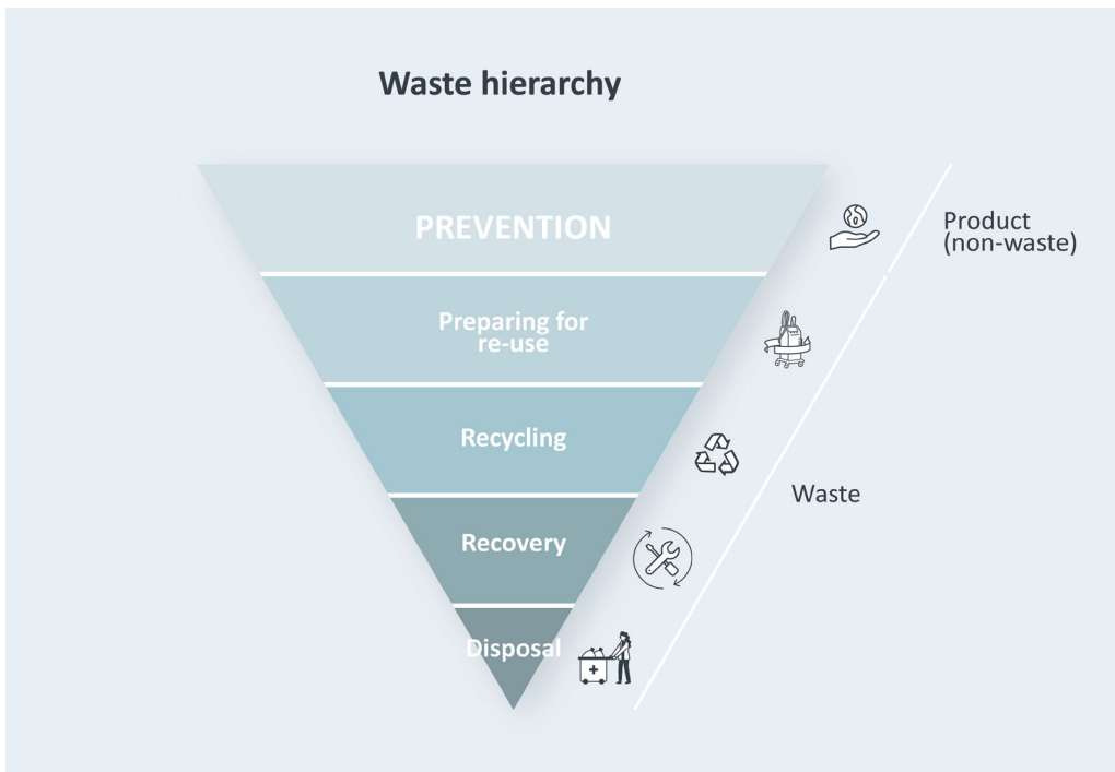
Figure 3.2: Waste hierarchy, adapted from the Waste Framework Directive by the European Commission (2008)
