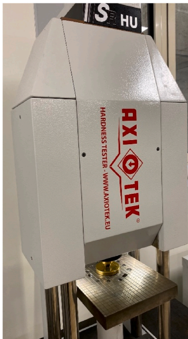
Fig. 4. The calibrated macro instrumented indentation platform ISRHU09 by AXIOTEK.
