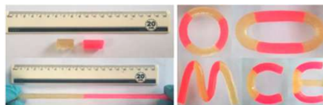
Figure 33. Upper Left: Self-healing between two colored hydrogel cylinders comprised of AA and \beta -CD grafted on maleic anhydride. Lower Left: Stretching properties of the repaired polymer. Right: Shapes and letters accessible from self-healing between multiple segments. Figure reprinted and adapted with permission from Ind. Eng. Chem. Res. 2019 , 58 , 3885–2892. 212 Copyright 2019, American Chemical Society.
