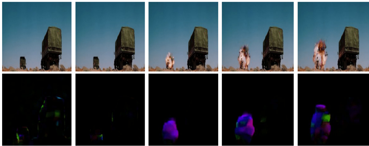
Fig. 1. Sequence of frames in RGB format and their corresponding optical flow. In this frame sequence, we go from a normal event to a violent event (explosion). Images from the XD-Violence dataset (Wu et al., 2020).
