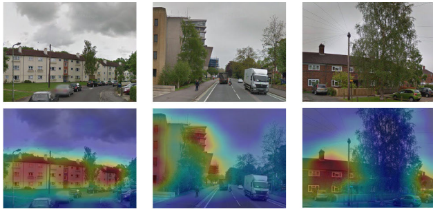
FIGURE 6. Examples of images from urban environment (top) and the attention scores (bottom) generated by the AdAGeo architecture [168] which implements attention via class specific activation maps. The attention is focused on building, disregarding dynamic objects, uninformative areas (sky) and objects that are not stable over time (trees).
